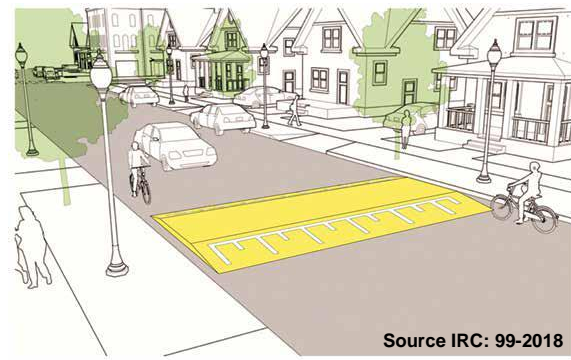
Figure 8 Trapezoidal Hump – Flat top with tapered sides
